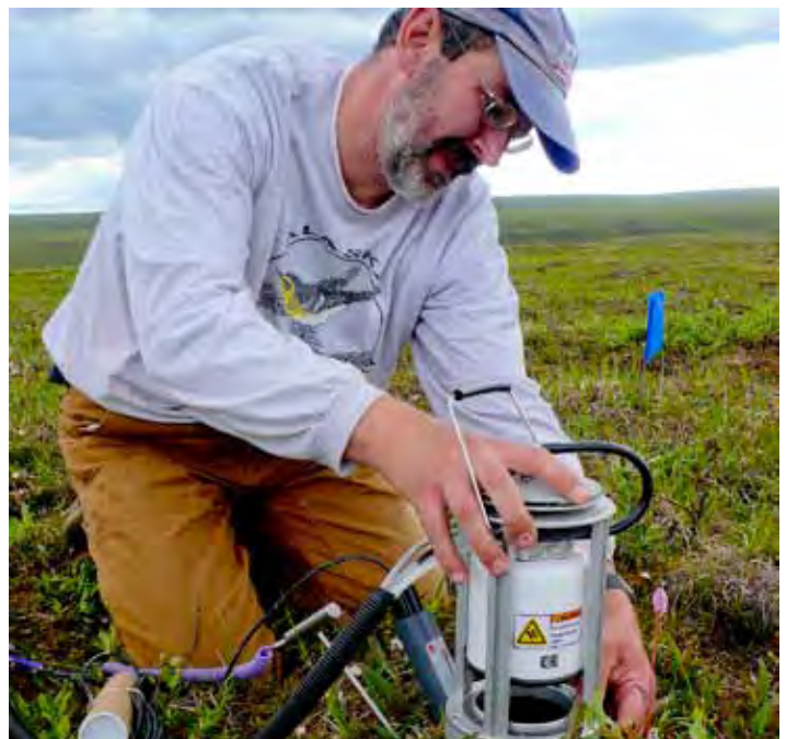
▼ Jay Jones attaches a gas flux chamber to a plastic collar marking a spot where he'll measure the carbon dioxide and methane outgassing from an undisturbed area of the tundra.
