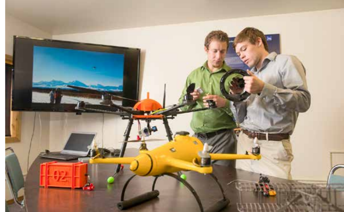
Sam Vanderwaal, left, and Corey Upton determine how to install a camera and a video transmitter in a drone payload extension module. The black drone with an orange top on the table is a Ptarmigan UAS designed by NES staff; the yellow drone is an H20Copter.
