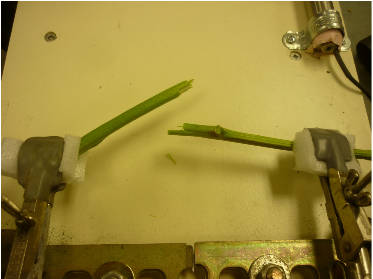
Plate 5. Peony stem was broken after imposed certain force with the force at the point of stem breaking recorded in the data logger.
