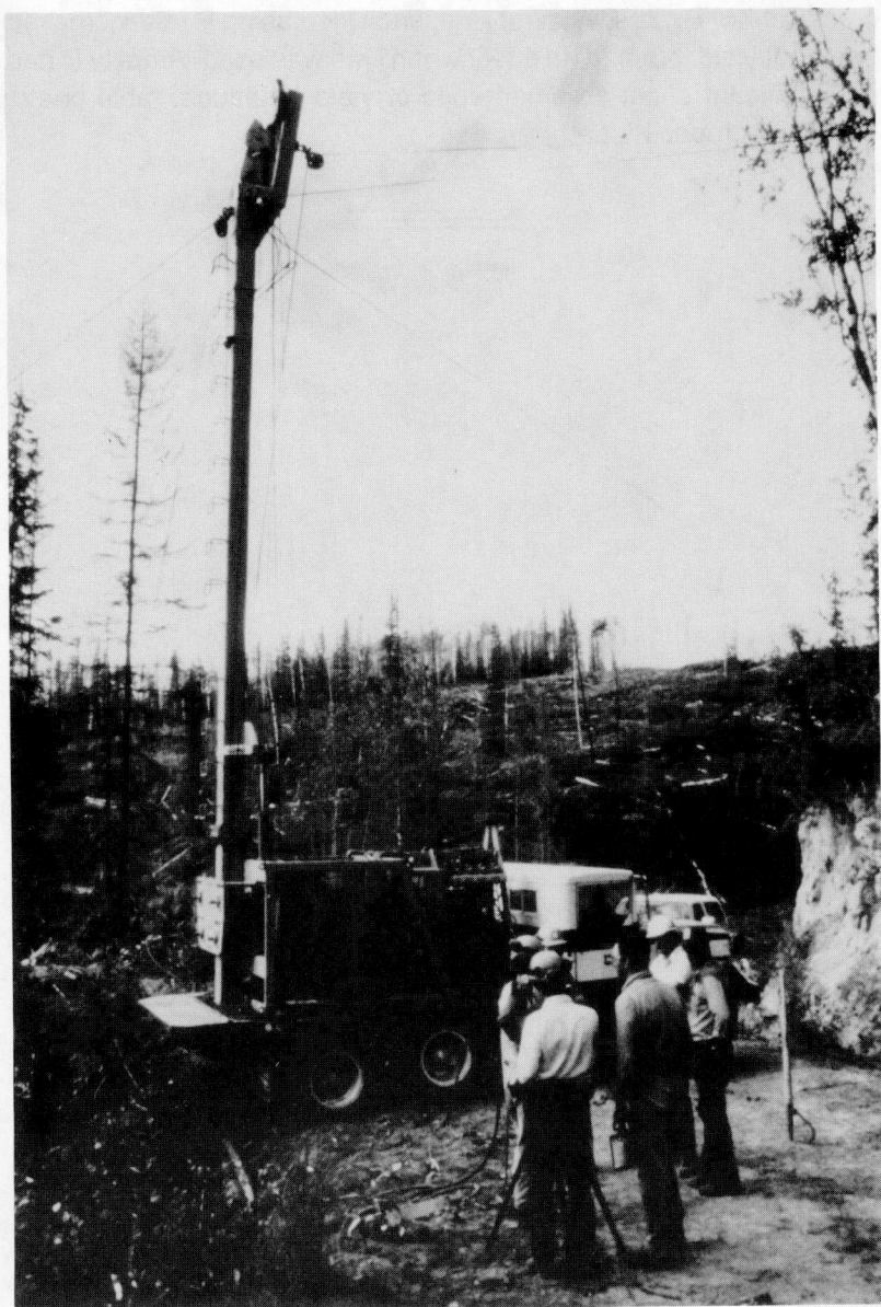
Development of timber-harvesting procedures emphasizing the use of a small cable yarder for interior Alaska forests is one goal of the Intensive Forest Management Project.
