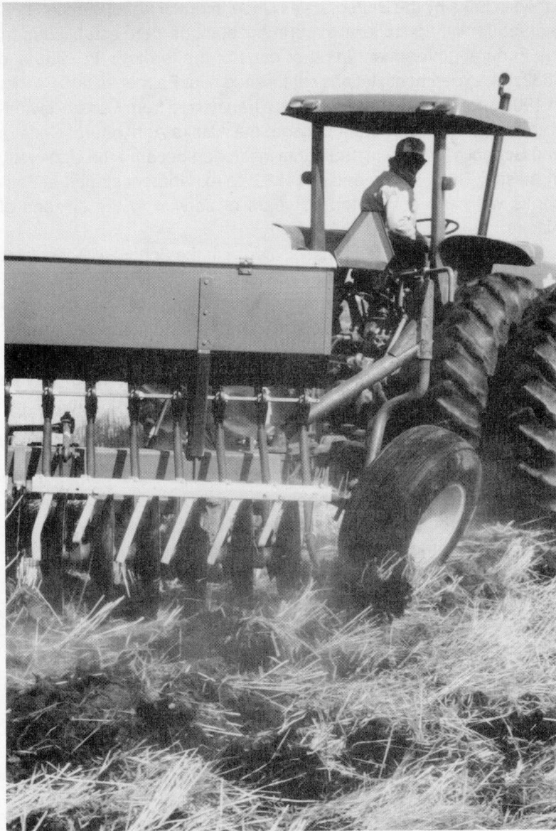
This one-pass disk/seeder is being used in research to find ways to enhance retention of soil moisture and improve weed control while, at the same time, reducing soil erosion by wind in the Delta Junction area of interior Alaska.
