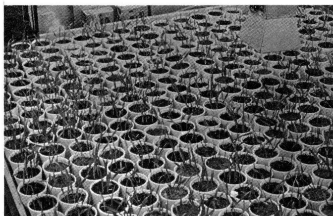
FIGURE 3. The interior of the growth chamber with the CaCO 3 incubation study in progress. The unit suspended above the work table in the upper right-hand corner is the heat and light sensor.
