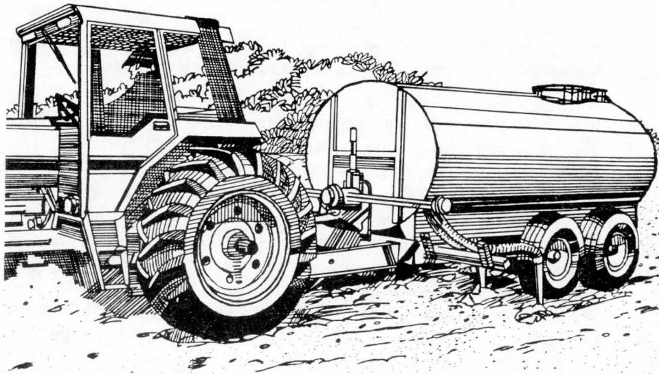
Figure 8. Side-mounted, adjustable, spring-loaded knives inject manure into the soil from the tankwagon.
