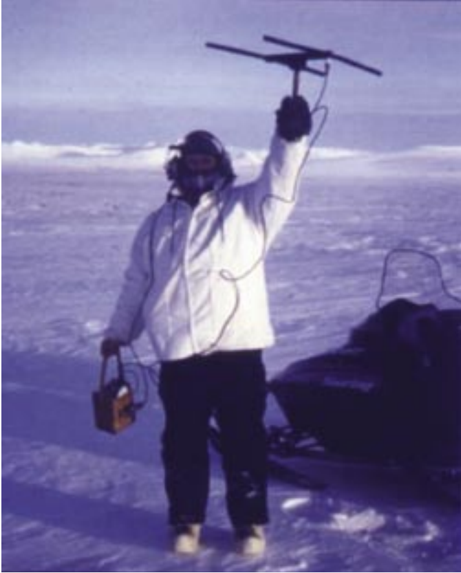
A biologist uses a receiver and antenna to locate a radio-collared reindeer on the Seward Peninsula.
