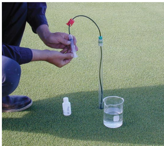
Left: Lysing sticks, also known as lysimeter tubes or soil solution access tubes, collect samples of fertilizer components captured from various root levels of the golf green's profile. Samples taken below root zones track any components that were not utilized by plant uptake.
