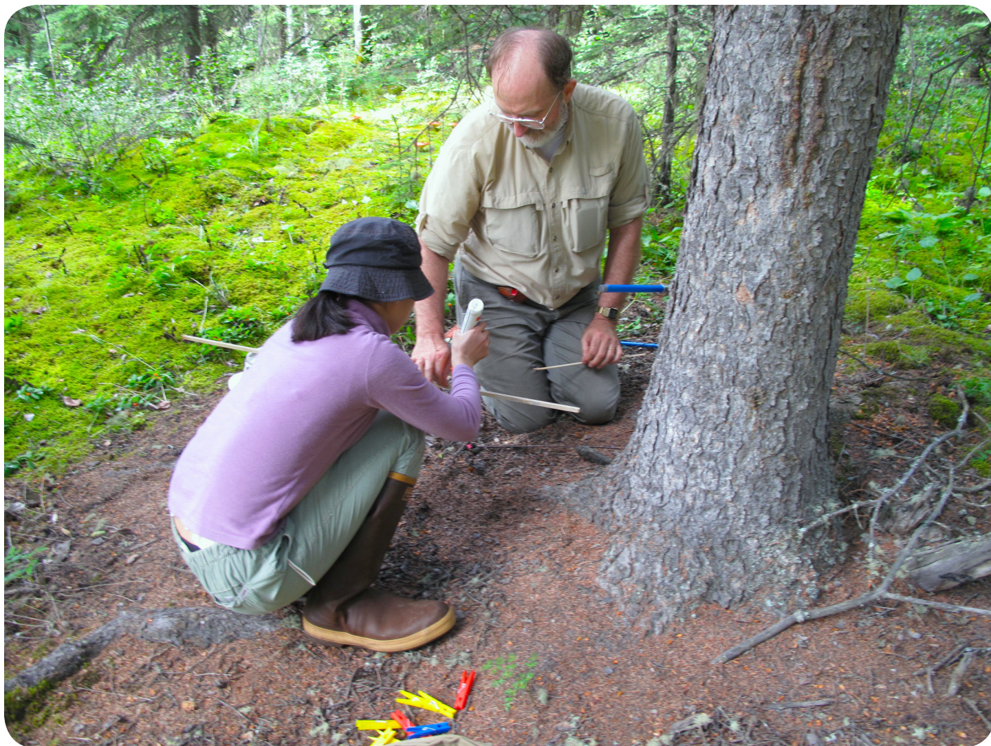
Author (Glenn Juday) with Japanese exchange student Miho Morimoto from Hokkaido University in northern Japan, Quartz Lake vicinity, near Delta Junction, Alaska, July 2010. Cores extracted from the drill-like corer (blue handle) provide a record of the tree's growth performance based on ring-width and the physical and chemical properties of the wood. This tree is about a century old, and registers increasingly unfavorable climate conditions in recent decades. Photo taken by David Klein.
