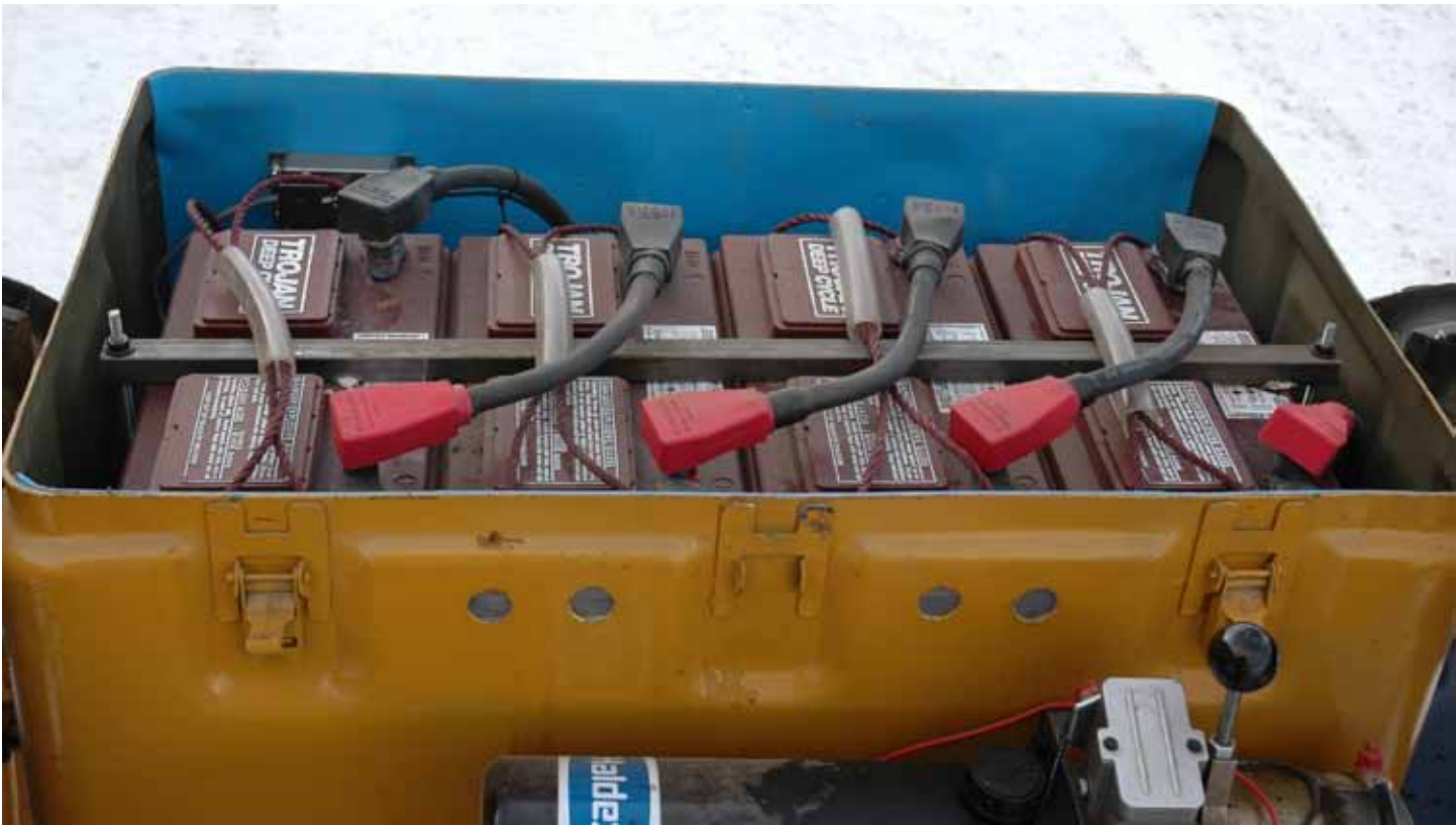
Photo E: side view of waterproof battery case.
