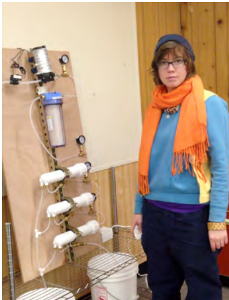
Tricia Kent, above, demonstrating her initial low-cost reverse osmosis unit. The vertical unit at center is a filter to remove debris; the three horizontal units contain the reverse osmosis membranes. A video showing how it works is available for viewing at http://snras.blogspot.com/2014/01/graduate-student-invents-diy-reverse.html .
