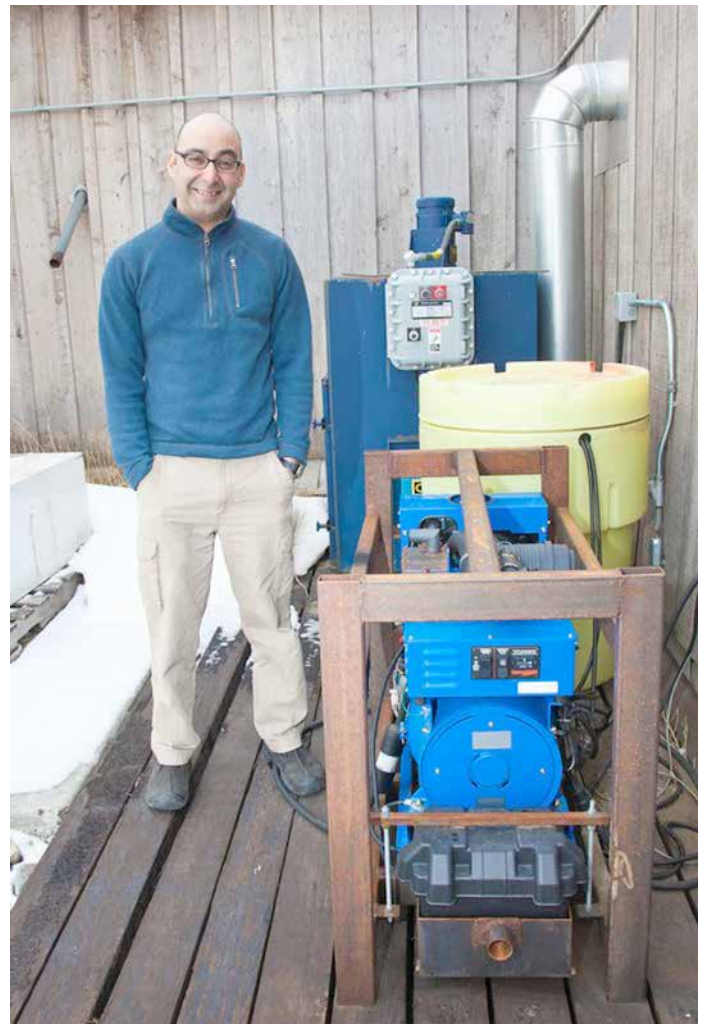
Andy Soria was a co-author on the 2011 National Academy of Sciences report, “Renewable Fuel Standard: Potential Economic and Environmental Effects of U.S. Biofuel Policy.” He is shown here in 2011 with a 6KW generator that burned the biofuel produced from the bio-oil experiments. The generator powered the lab in Palmer.
