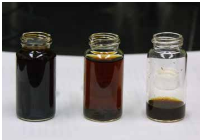
Bio-oils made from different Alaska trees, using supercritical fluid liquefaction. Left to right: birch, alder, and Sitka spruce.
