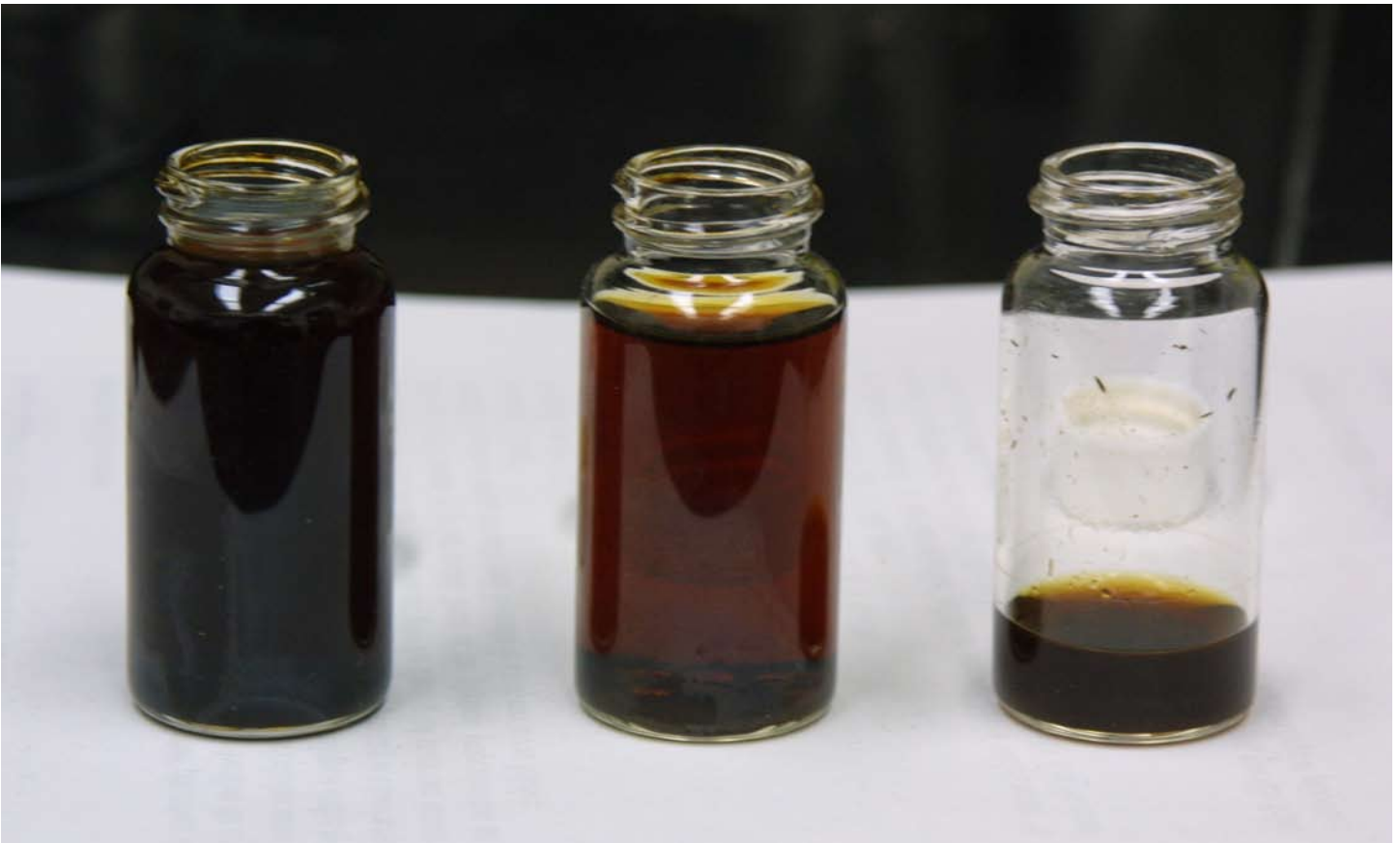
Three different bio-oil extracts, from birch, alder, and Sitka spruce, created using supercritical fluid liquefaction of woody biomass. —PHOTO BY J. ANDRES SORIA
