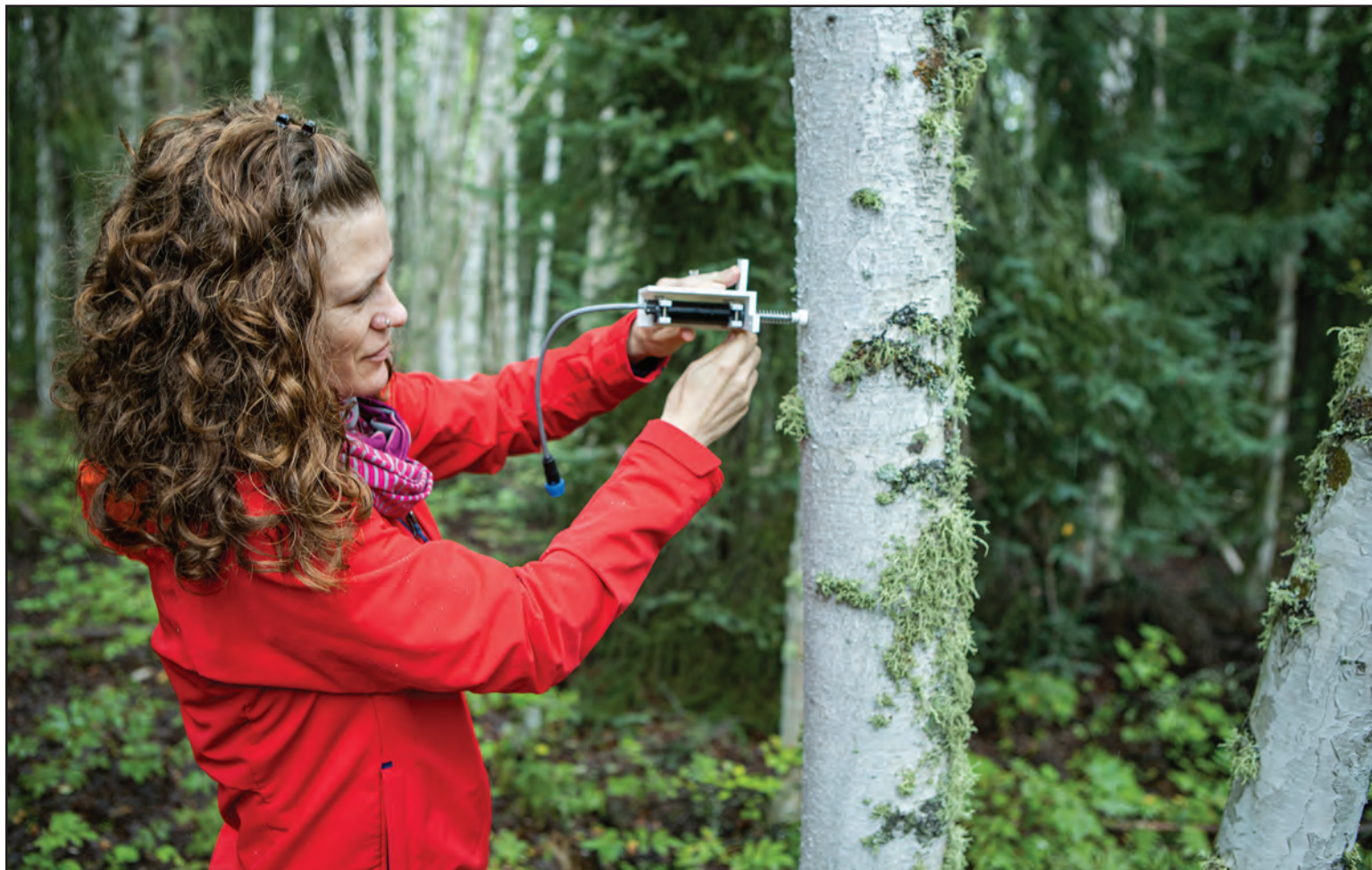
Jessie Young-Robertson is researching the seasonal variation of water content in trees to determine the best time to harvest firewood. She demonstrates a device for measuring moisture content. UAF photo by J. R. Ancheta.
