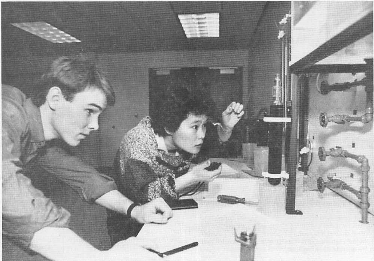
Paul Wahnoutka looks on as Hyun Park measures the speed of a ball bearing passing through a glass cylinder. This is one of many experiments performed by students in the Fluid Mechanics Laboratory, located in the new addition to the Duckering Building.
