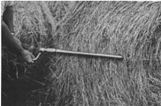
Figure 3. Sample round bales with a core sampler and insert at right angle to the wrap.
