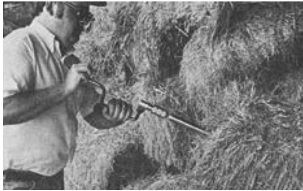
Figure 2. When using a core sampler (such as the Penn State Forage Sampler), insert into the end of conventional bales to get the best cross section of leaves and stems.
