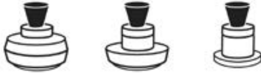
Above, a three-piece pressure Presto regulator. At left, a 15-pound Presto pressure regulator (or "dead weight.")
