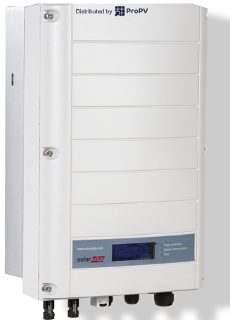
Figure 12. The SolarEdge central, or string, inverter shown here measures about one foot wide and two feet tall. This particular inverter model utilizes DC optimizers at each panel to optimize power output. Source: www.propv.eu/
