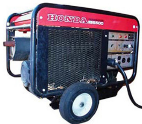
A typical generator similar to many that are used for off-grid PV systems is shown above.
