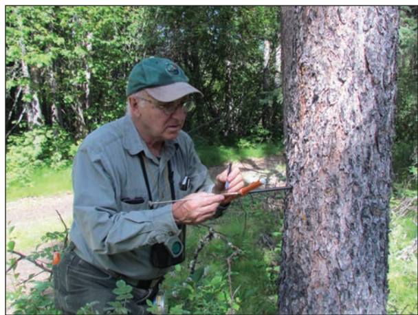
An increment borer is used to determine a tree's age and growth rate.
