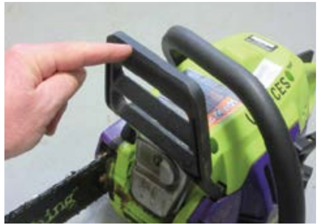
The chain brake indicated above is found just in front of the top left-hand chainsaw handle.
