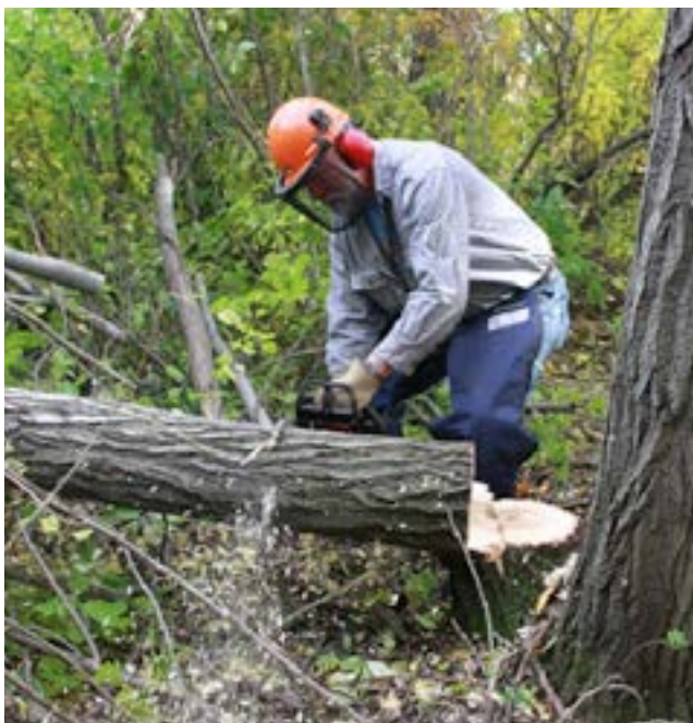
... and finished from beneath to avoid the chainsaw bar becoming pinched.
