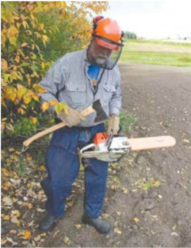
Use a hard hat, eye and ear protection, protective chainsaw chaps, tough gloves and protective footwear whenever operating a chainsaw.
