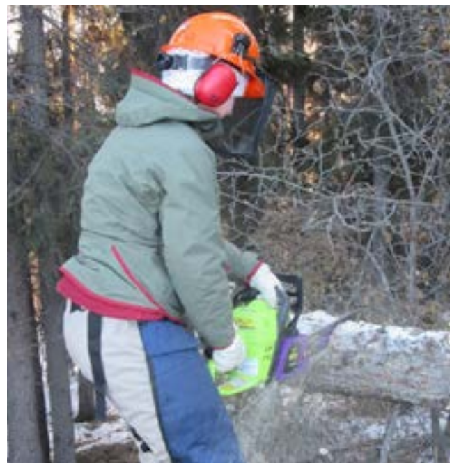
Hold the chainsaw firmly and keep it close to the body to give you better control and less fatigue.
