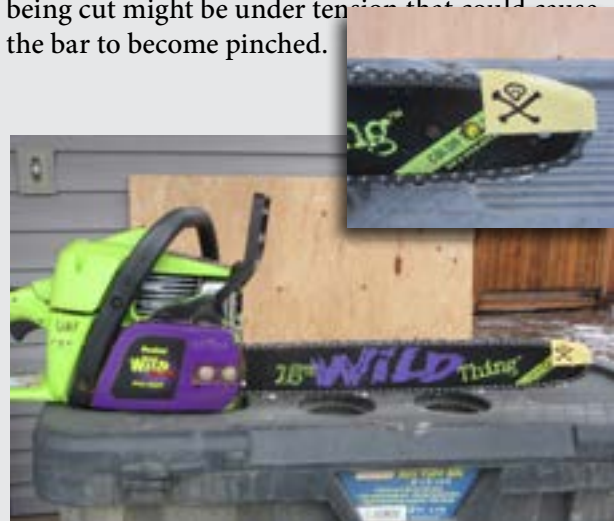
Kickback occurs when the top tip of the running saw contacts a solid object. Note the yellow tape on the kickback zone of the chainsaw bar.
