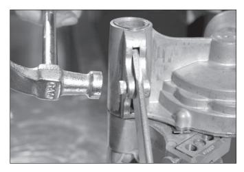
Insert the lever pivot from the back — knurled (ridged) side of the pivot out. Tap in the lever pivot with a hammer.
