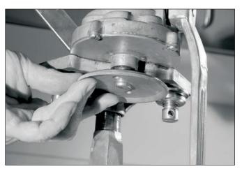
Rotate the crank until the "0" appears in the indicating window. Select the appropriate chuck for the can size you will be using (see page 5). With the concave face of the chuck facing down, insert the chuck screw through the center of the chuck. Thread the screw into the head by hand. Do not use a screwdriver.
