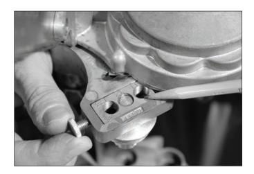
Rotate the crank until a "2" appears in the indicating window. Install the second seaming roller on the left side in the same manner as the first (see steps 1-3). Note the orientation of the 3-hole nut (pencil points to the #1 hole).
