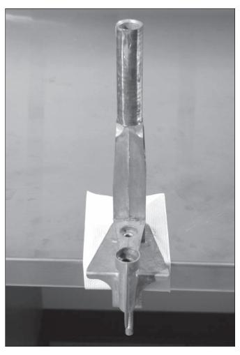
Start by clamping the frame securely to a table. Use the 3-inch pin to tighten the clamp screw. Use a cloth or a piece of cardboard to protect the surface of your table.
