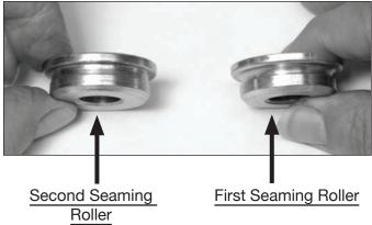
There are two seaming rollers. The "first" seaming roller is on the right side of the sealer and is for curling the lid and can body edges together. This roller has a deeper, more rounded profile.
