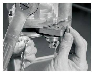
Make sure that the "1" appears in the indicating window. Insert the **THICK/LARGE** gauge wire between the chuck and the groove in the first seaming roller.
