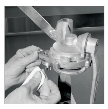
Make sure the "2" appears in the indicating window. Insert the **THIN/SMALL** gauge wire between the chuck and the groove in the second seaming roller.
