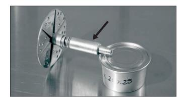
Select the required spacers and extension for your can size (see page 5). Place the spacers, then the spring onto the shaft of the turntable. For the 307 x 200.25, ¼-pound flat salmon can, the turntable extension is required (arrow).
