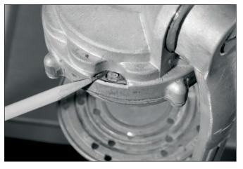
The second seaming roller is on the left. Turn the crank clockwise until the "2" appears in the indicating window. You will see a "C" pass before the "2" appears in the indicating window (pencil point in photograph).
