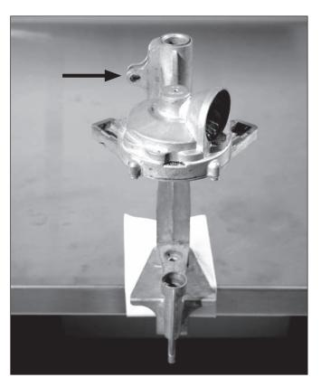
The head drops onto the frame. Notice that there is a slot in both the head and in the post of the frame (arrow).
