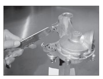
Place the head on the frame post. Align slot in the head with the slot in the frame. Insert the lever into the slot (writing should face forward). Line up the hole in the lever with the two holes in the head.
