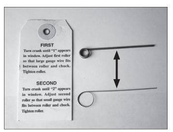
Accurately setting and securing both seam rollers is essential. The first and second gauge wires are used to set the distance between the rollers and the chucks. These settings control the shape and tightness of your can seams and, therefore, the quality of the hermetic seal. Since food must never be stored in cans that have improperly formed seams, an improperly adjusted can sealer has no role in food preservation.
