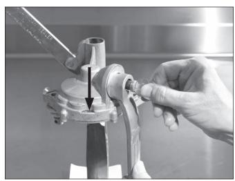
Finger tighten the screw. Turn the crank handle until the "0" appears in the center of the indicating window (arrow).
