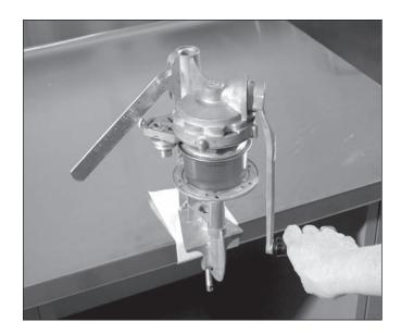
Steadily rotate the crank clockwise through the entire cycle, starting and ending at "0" in the indicating window. The indicating window will display "0," "1," "C," "2" - then back to "0" in a complete can seaming operation.
