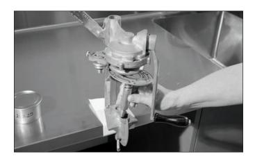
Situate the turntable by lifting the can sealer lever to the up position. Insert the turntable into the frame.
