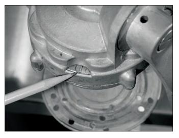
Turn the crank clockwise until the "1" appears in the indicating window, as indicated by the pencil point in the photograph. The crank should again be hanging straight down.
