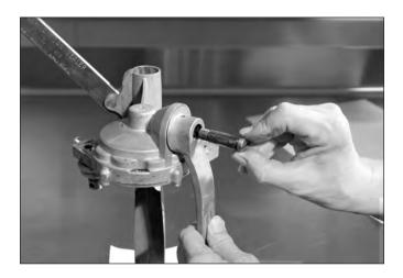
Insert the gear end of the crank into the head. Thread the screw.
