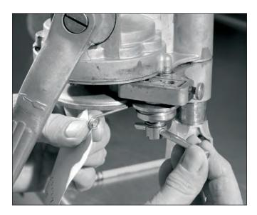
Lock the seaming roller screw in place by tightening with the 3-inch pin. Draw (lightly pull) again on the gauge wire — it must not move easily. If it moves, loosen the seaming roller screw slightly, and tighten the thumbscrew slightly. Repeat until the gauge wire cannot be moved easily.
