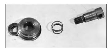
Make the first roller assembly by putting the spring onto the roller screw, then the seaming roller and then the washer. The largest part of the seaming roller is next to the washer.
