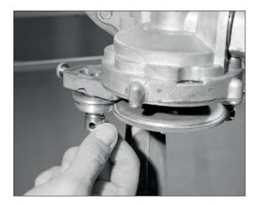
Move the seaming roller to the outside by sliding the 3-hole nut until it stops hard against the frame.
