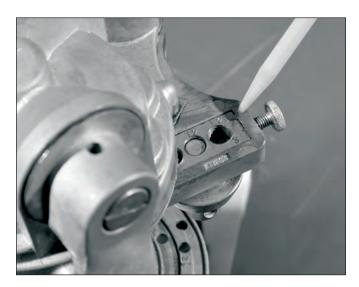
Back out the thumbscrew and slide the first seaming roller and 3-hole nut to the outside, hard against the frame (pencil point in photograph). The first roller is to the right.
