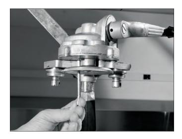
Insert the 3-inch pin into one of the small holes in the chuck. Turn the crank clockwise until the 3-inch pin is pressed against the frame and chuck is tight. Remove the pin.
