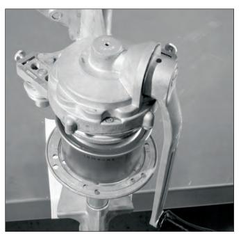
Begin with the "0" in the indicating window and the crank hanging straight down. Raise the lever to the full up locked position. Center a can on the turntable, then center a lid (gasket down) on top of the can.
