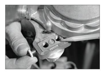
Rotate the crank until a "2" appears in the indicating window. Install the second seaming roller on the left side in the same manner as the first (see steps 1-3). Note the orientation of the 3-hole nut (pencil points to the #1 hole).
