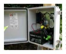
Dataloggers store the numerous measurements of soil-water content collected by electronic sensors. Data can be downloaded with a laptop or accessed by a remote computer. Computer software programs are necessary to organize and interpret the measurements so that you can use the data to make irrigation decisions.
