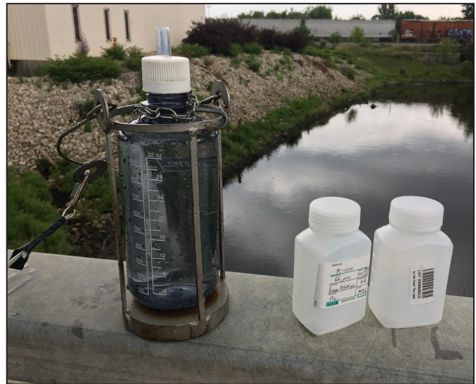
Two water samples to be tested for PFAS are taken from Portage Creek, in the Kalamazoo River watershed. Photo by Michigan Department of Great Lakes, Environment and Energy
