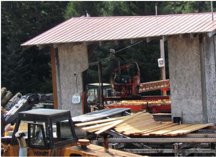
JK has an electric Mobile Dimension "mega mill" model circular sawmill which will increase lumber volume output. Glen Holt photo
