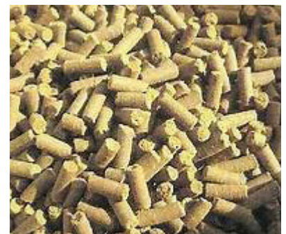
Utilizing wood thinned during fuels reduction programs might include manufacturing wood pellets for home heating fuel.
