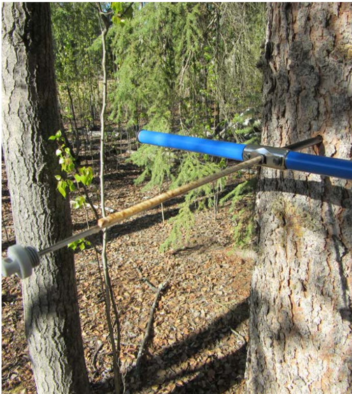
An increment bore is a tool used to measure the growth rate increment within a set number of years and/or the age of the tree by counting growth rings.
