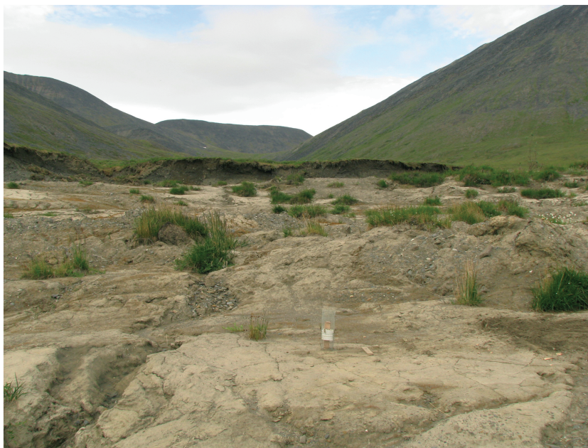
Figure 2. Retrogressive thaw slump in the upper Nigu Valley. Data-logging station in foreground. Active thaw face in background with intact moist acidic tundra and soil surface organic layer (SSOL) beyond. Temperature logger and radiation shield is enclosed in a cage of hardware cloth to deter animal disturbance.
