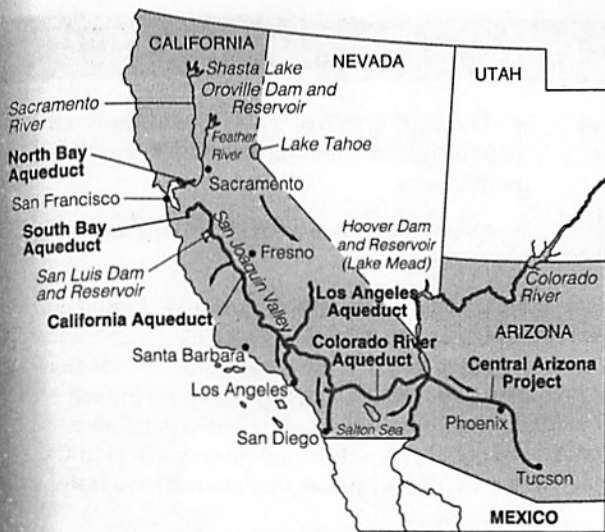
Figure 14-13 The California Water Project and the Central Arizona Project involve large-scale water transfers from one watershed to another. Arrows show the general direction of water flow.
