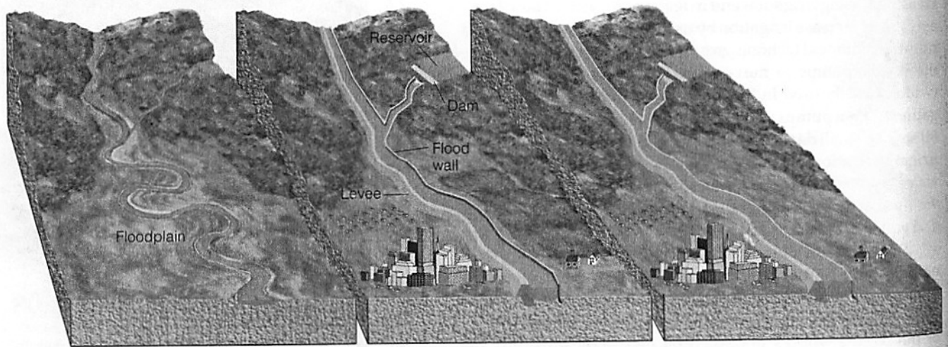
Figure 14-22 Land in a natural floodplain (left) often is flooded after prolonged rains. When the floodwaters recede, deposits of silt are left behind, creating a nutrient-rich soil. To reduce the threat of flooding (and thus allow people to live in floodplains), rivers have been (1) dammed to create reservoirs that store and release water as needed, (2) narrowed and straightened (channelization), and (3) equipped with protective levees and walls (middle). These alterations can give a false sense of security to floodplain dwellers living in high-risk areas. In the long run, such measures can greatly increase flood damage because they can be overwhelmed by prolonged rains (right), as happened along the Mississippi River in the midwestern United States during the summer of 1993.
