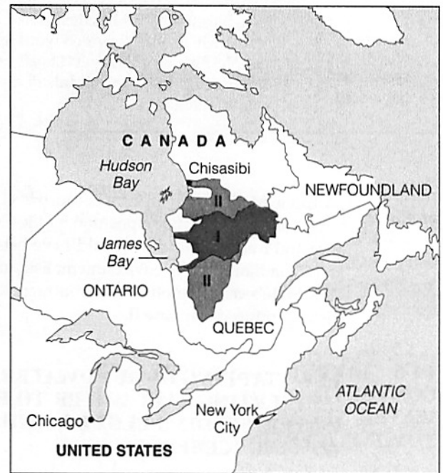
Figure 14-14 If completed, the James Bay project in northern Quebec will alter or reverse the flow of 19 major rivers and flood an area the size of the state of Washington to produce hydro-power for consumers in Quebec and the United States, especially in New York State. Phase I of this 50-year project is completed.
